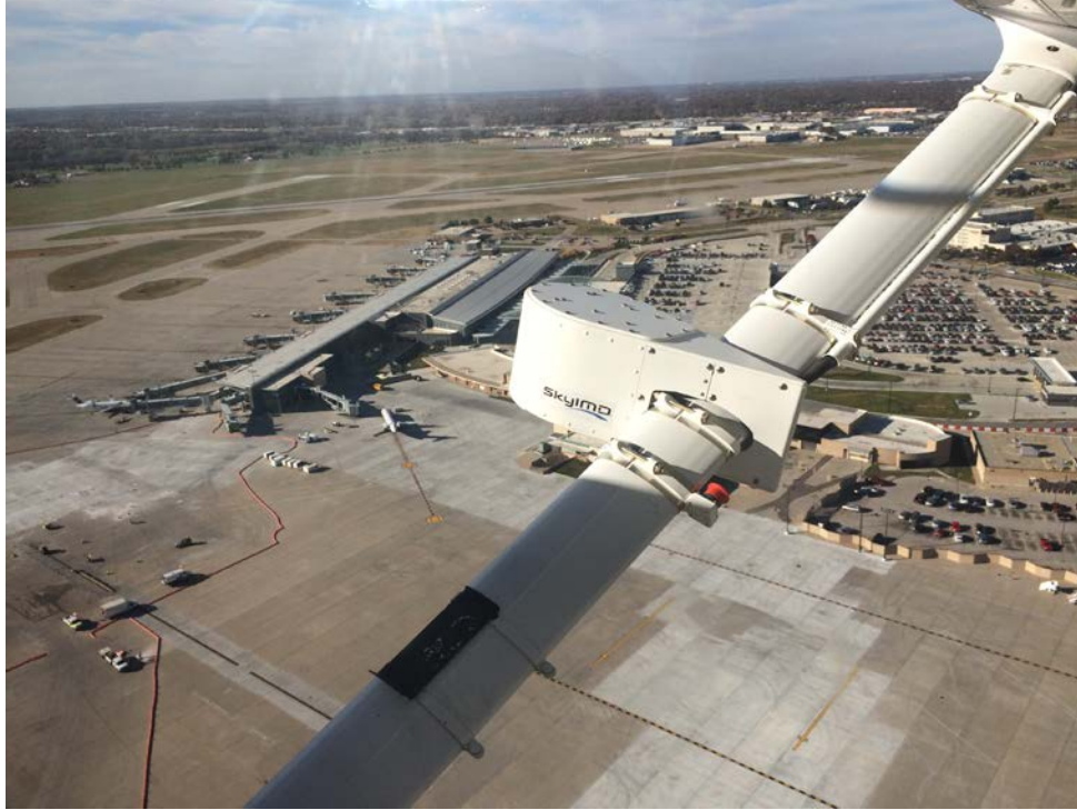
Figure 2. Sensor Pod Mount on the C172S Wing Strut
