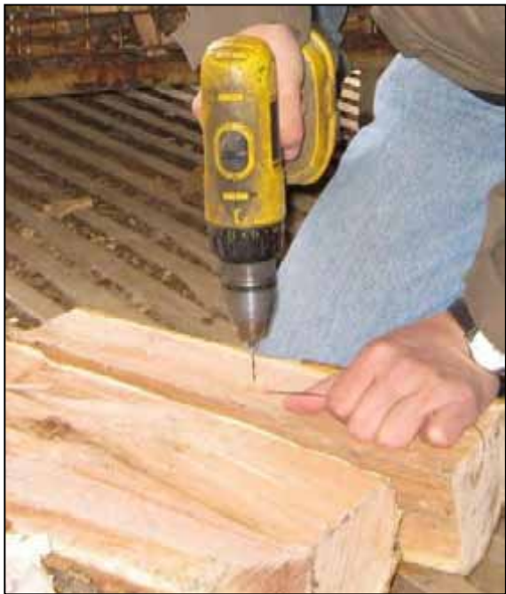
Figure 4.13. ~ Drill a hole in the firewood to accommodate a temperature sensor. Drill a hole from the side at midsection for a thermocouple (left). Drill a hole from the end for a probe (right).
