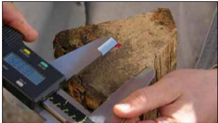
Figure 4.12. ~ Locate the center of the firewood from the end.
