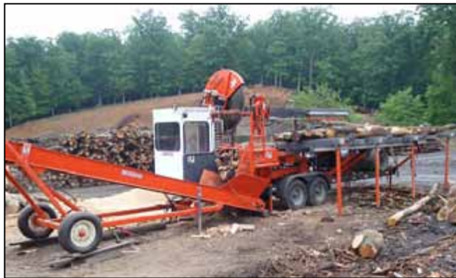
Figure 3.17. ~ High production firewood processing equipment. Photo courtesy of Multitek North America LLC.
