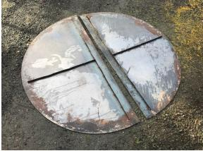
Above left: Use three clamps for each join. Space clamps evenly. Above right: The kiln lid is in 2 pieces. Place down inside the kiln on top of hot char and make sure that the center sections overlap. Seal the rim with dirt.
