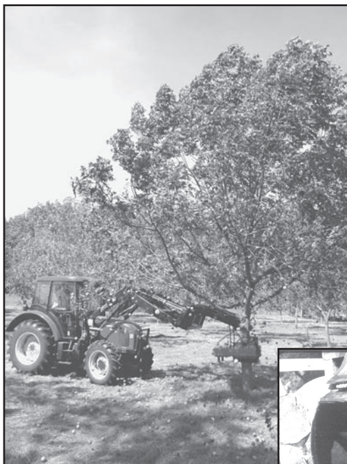
Fig. 13. (Left) A tree shaker mounted to a front-end loader is used to remove walnuts from the tree. Fig. 16. (Right) The tire and cage huller uses the force of a rotating tire to smash the hull against a rebar cage, removing hull from nut. Fig. 17. (Below) A homemade nut washer features rubberized stirring paddles. Fig. 18. (Below right) Nuts are spread on drying racks and allowed to air dry.
