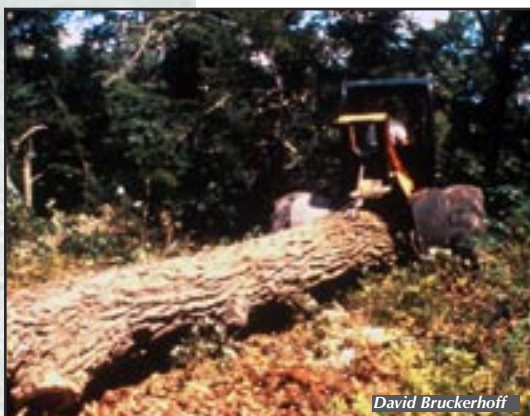
Skidder moving harvested logs from woods to truck loading site..
