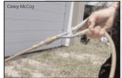
A quick connect coupling makes changing from attachment to the blower to the normal spray wand an easy job.
