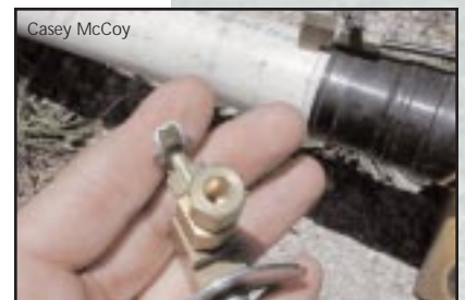
Installation of a valve in the discharge tube lets the operator control the amount of water introduced into the air stream.
