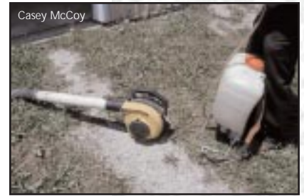
The system uses two well recognized hand tools — a gas powered leaf blower and a back pack pressure pump.
