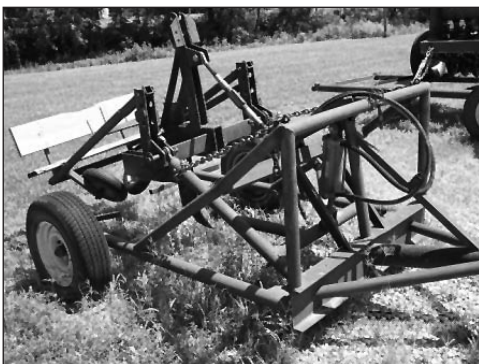
This is another version of a root plow on a trailer.
