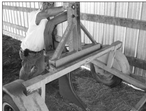
The plow rotates vertically and is lifted off the trailer using the three-point hitch.
