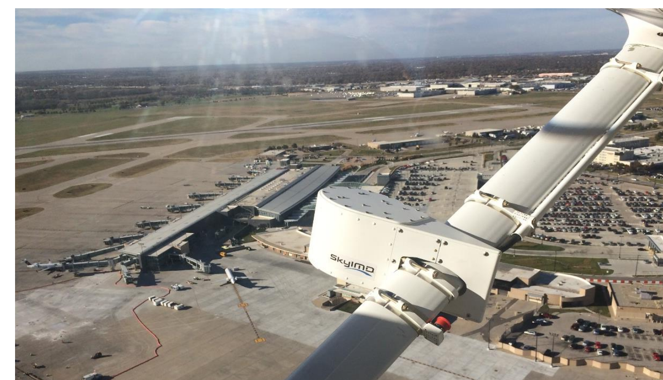
Sensor pod mount on the Cessna 172S wing strut
