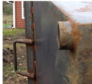
Handle and drain hole details of the Oregon Kiln.
