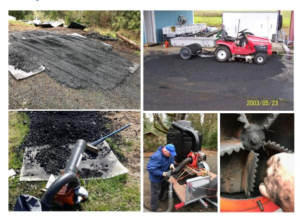
Biochar can be crushed by driving over it with a truck or lawn roller. A small leaf vacuum works fairly well, but a large one is much better, with a more effective and durable impeller for chopping char. You can also use a hammer mill or a roller mill. Be aware that dry char can be very dusty and that wet char can stick and clog machinery. Experiment with moisture levels to find the sweet spot for the equipment that you use for crushing.
