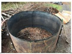
Set up the heat shield. Load the initial charge – loosely packed.
