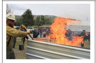
Wear fire-resistant clothing, and use a heat shield around the kiln.
