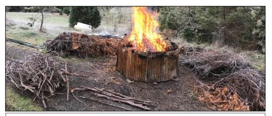
For safe and efficient production, place the kiln in a clear open area and stage your feedstocks nearby, but not too close. It helps to sort material by size.
