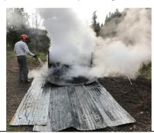
Dry quench method – place cap, seal edges with dirt. Check that bottom is sealed too.
